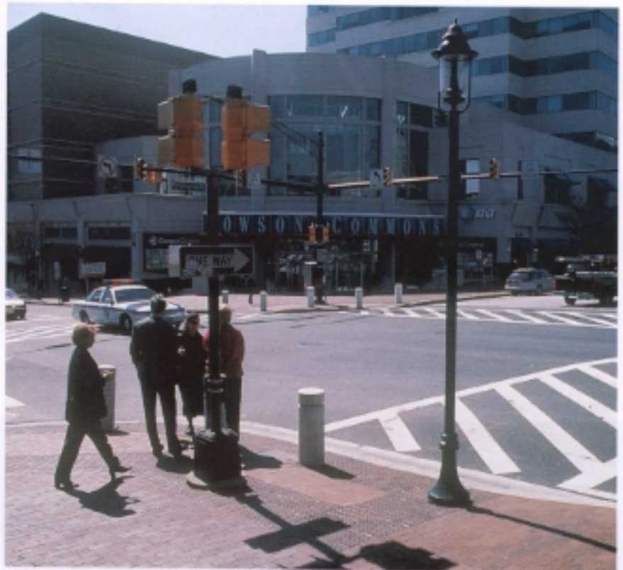
Baltimore County Public Works' streetscape plan extended the amenities and landscaping treatments from the roundabout westward into the center of town, where they slow the approach of traffic into the circle, while stimulating renewed foot traffic for local businesses.
